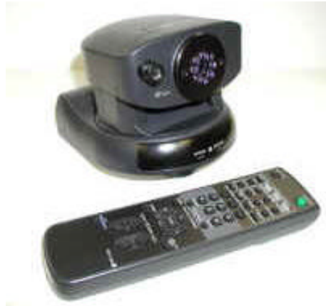
Figure 2: . Infrared Camera of the Eye Gaze Tracking System used to measure the pupil diameter
