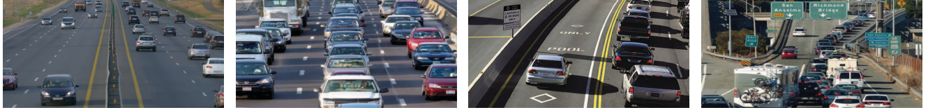
(a) Uniform traffic speed with low congestion (b) Uniform traffic speed with high congestion (c) Nonuniform traffic speed for carpool lane (d) Nonuniform traffic speed for highway exit
