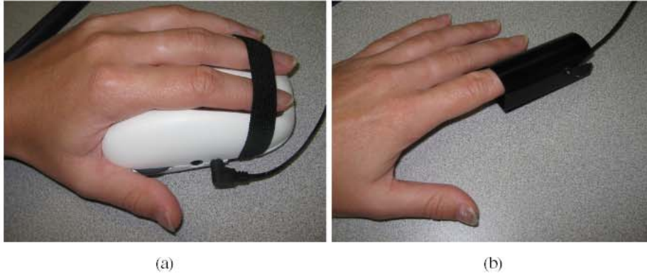
Fig. 1. (a).The GSR2 skin conductance device (Thought Tech LTD) (b). Pulse Plethysmograph.
