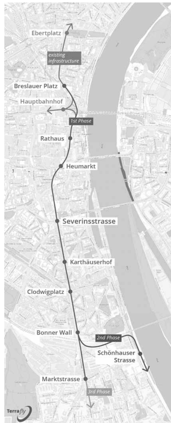
Figure 1: Planned route of Cologne's new subway tunnel, stations, interconnections, and line routes.
