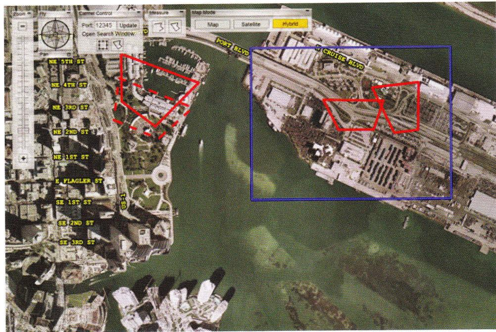
*CARMEL-TerraFly user interface. The map shows the Port of Miami with moving traces of areas videotaped by airborne cameras. Solid trapezoids are ground projections synchronized with playback and dotted trapezoids are real-time projections of camera views. The blue rectangle allows selection of video fragments at times and locations of interest.*
