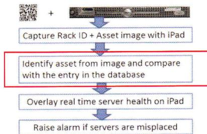
*Visual identification of computing assets for efficient data center operations*
