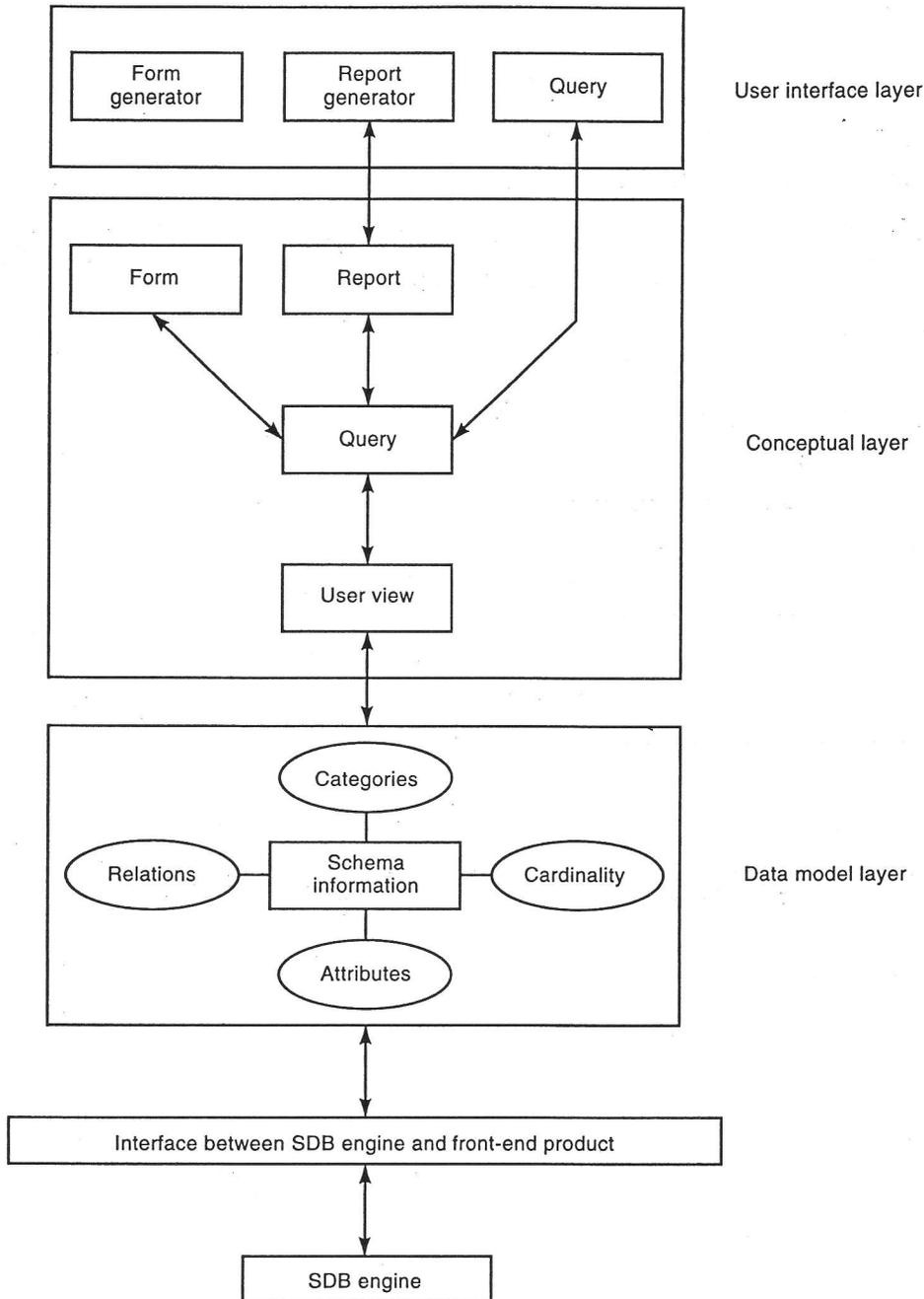
**Figure 2.** Architecture of the front end of SDB.
