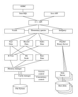
Figure 2. Sem-ODB Engine architecture
