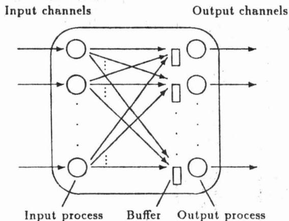
Figure 1: A sample node of a hypercube
