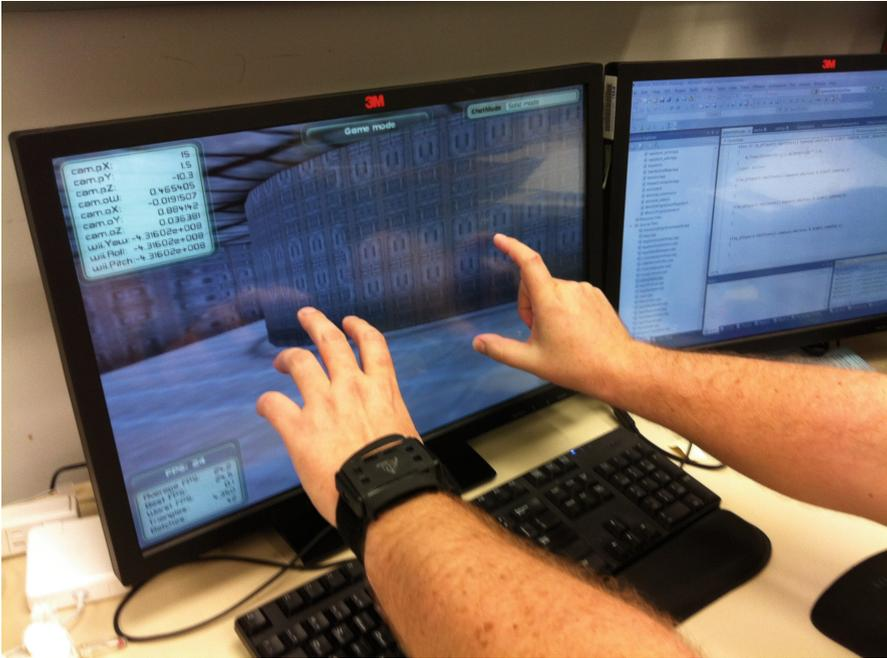
**Fig. 3.** 3M multi-touch display and gyroscope (left wrist)
