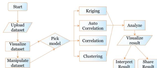
**Figure 3: The Workflow of TerraFly GeoCloud Analysis**
