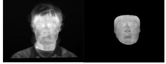
Fig. 3. Results of the segmentation process showing the original thermal image and the face segmented image.
