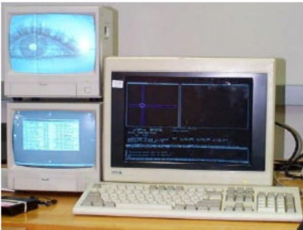
Figure 4. EGT system showing eye image processed
