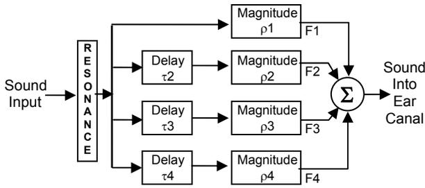
Fig. 2. Block diagram of pinna model (for 4 components).
