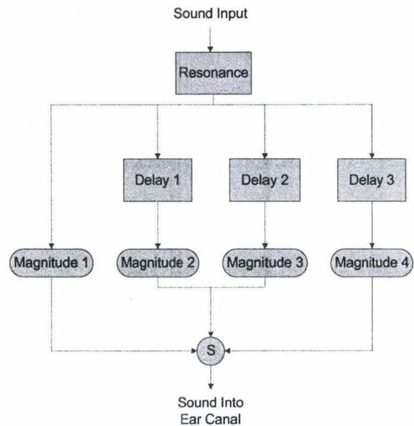
Fig. 2. Block diagram of pinna model (for 4 components).
