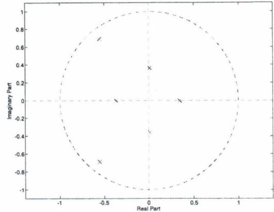
Fig.6: Poles obtained from the sixth-order STMCB approximation of the complete sequence  $x$ .
