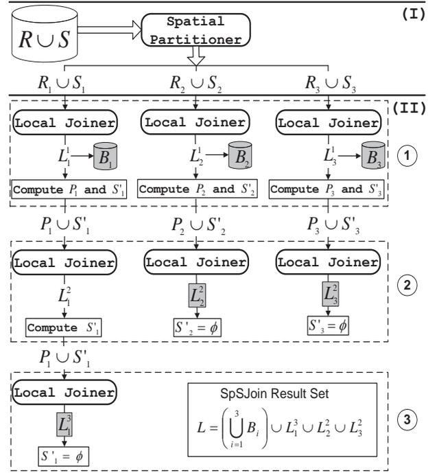
**Figure 5: Example workflow for SpSJoin.** *Spatial Filtering* phase is shown in step (I). The *Expansion* phase (II) performs iterations 1-3.
