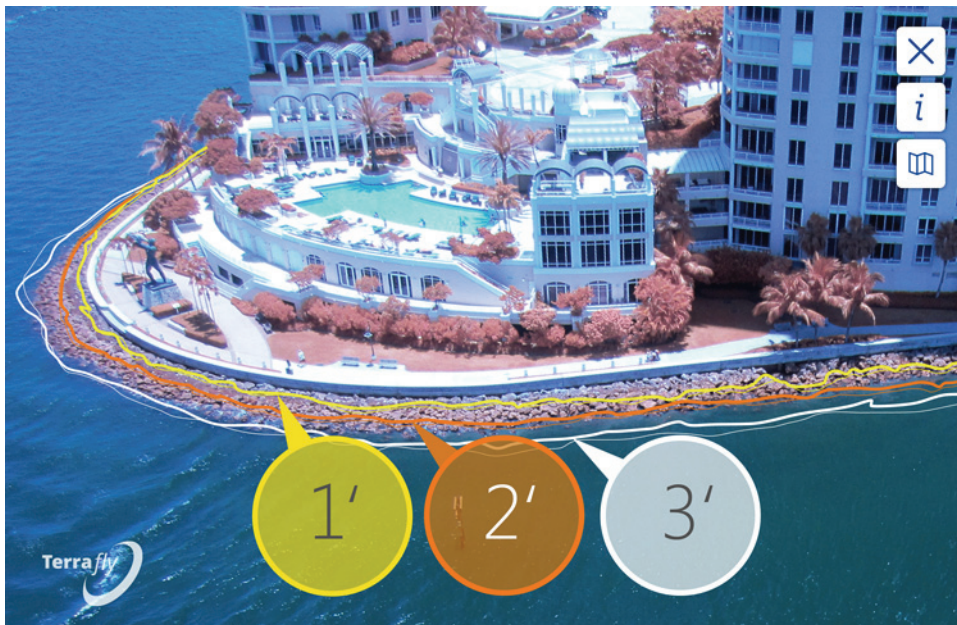
TerALTA balloon oblique multispectral aerial image, vegetation index in reddish color, derived nearshore sea depths and isobaths for NSF IUCRC Compendium CAKE-MSS Modeling Sea Surge and Flooding using ALTA and TerraFly. Image provided by CAKE.
