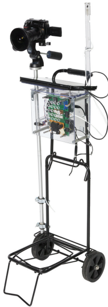
NEAT portable sensors and datalogger suite
