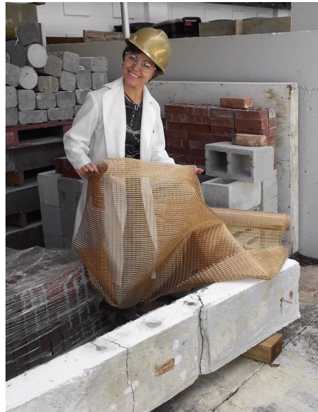
Fabric reinforcement for a concrete surface.
