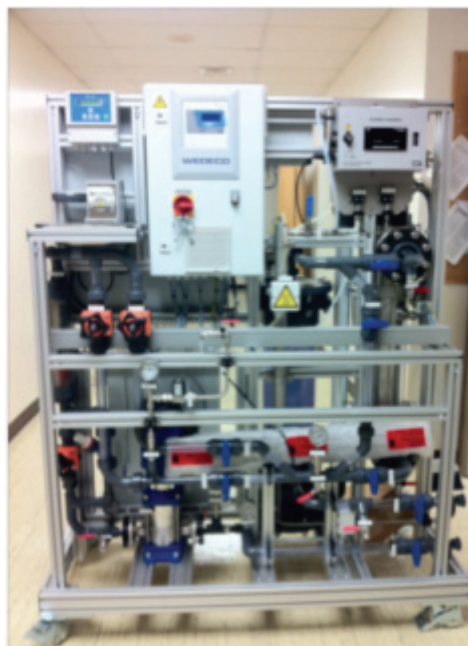
This unit is equipped with inline ozone monitors to measure ozone in air, water and atmospheric phase, a UV sensor, a degassing unit and a catalytic ozone destructor.
