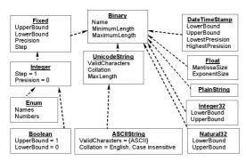
Figure 1: Sub-schema of concrete types
