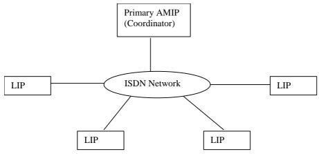
Fig 1.1 - Physical Architecture of QDA
