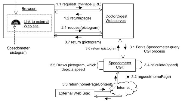
Figure 2. Speedometer module collaboration diagram.
