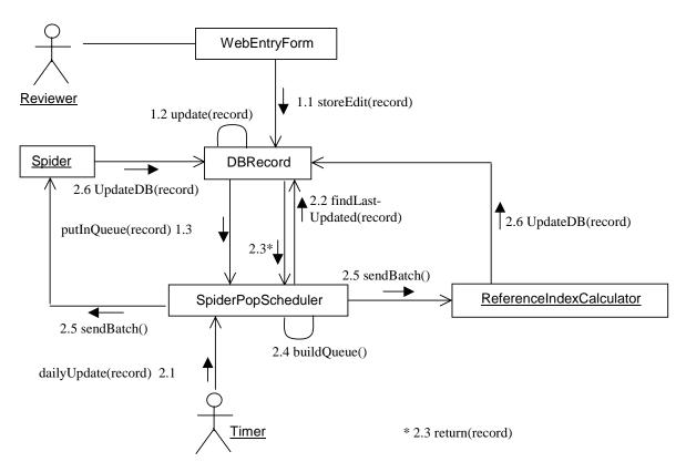
Figure1. Reference index calculator collaboration diagram.
