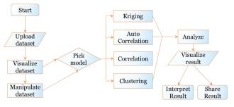
Figure 3: The Workflow of TerraFly GeoCloud Analysis
