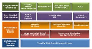
Figure 2: The Architecture of TerraFly GeoCloud
