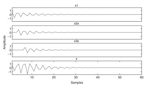
Figure 6. Plot of the three damped sinusoids (x1, x2s with delay  $\tau_2$  and x3s with delay  $\tau_3$ ) and the sum of them (x).
