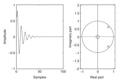
Figure 5. Time domain and zero-pole plot of a single second-order damped sinusoidal.
