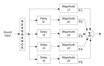
Figure 2. Block diagram of the pinna model.
