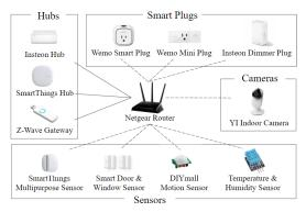
Fig. 1. The architecture of our data collection environment that is comprised of 11 different IoT devices.
