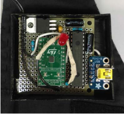
Fig. 1. Assembled hardware. (Image shows top-side view of assembled hardware with container and glove.)
