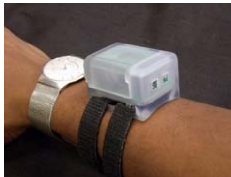
Wearable wristwatch-sized sensor used for robot-assisted stroke rehabilitation. Credit: Dr. Eric Wade.
