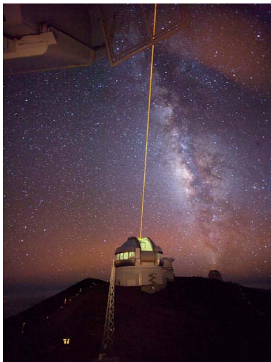
The Gemini North telescope photographed while propagating its guide star laser. The laser excites neutral sodium atoms at a height of about 90 km in the Earth's atmosphere, which produces an artificial guide star which is used by the adaptive optics system to correct for the blurring of the atmosphere. Credit: Gemini Observatory.
