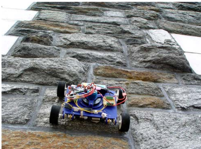
CityClimber prototype-IV on a brick wall. Credit: Umit Uyar and Jizhong Xiao, CUNY City College of New York.
