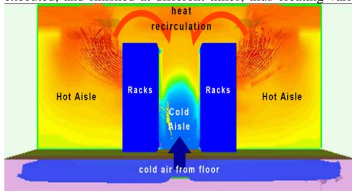
Figure shows the heat recirculation effect in a typical data center using a cold aisle – hot aisle configuration. Credit: Image generated in the Arizona State University Impact lab using the Flovent Computation Fluid Dynamics (CFD) software.
