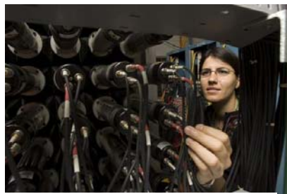
A NSCL research associate adjusts cabling on a detector. Credit: NSCL.
