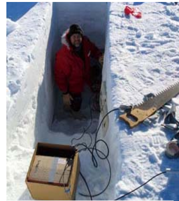
Trench in which seismometers were deployed on iceberg C-16. Credit: Tim Parker.
